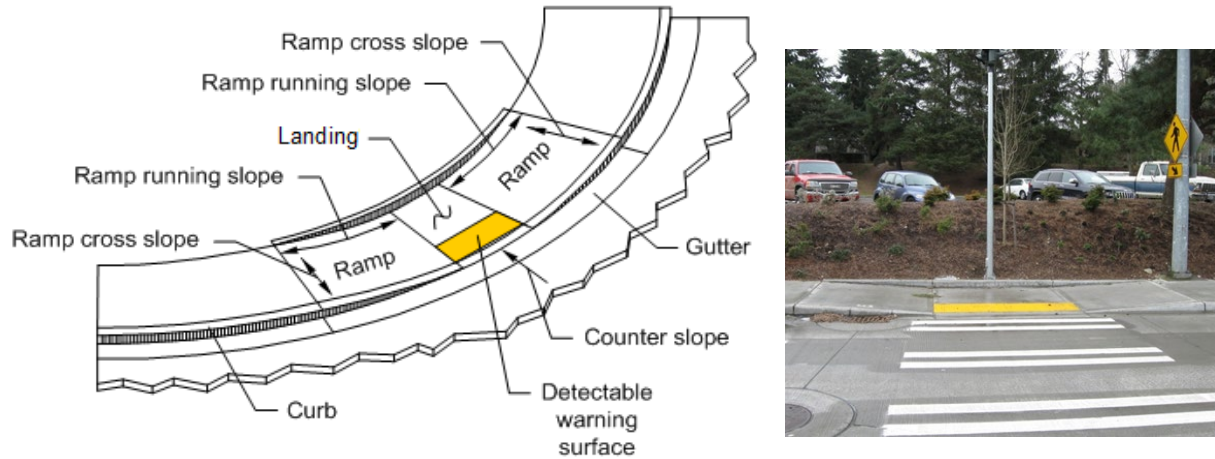
Figure 8-3: Parallel Curb Ramp Common Elements
